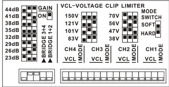
**VCL-Voltage Clip Limiter** adjustment is provided for eight discrete levels for each channel. Select the setting most appropriate for connected speakers.
