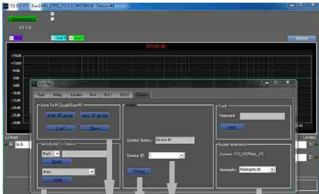
PRESET SAVE OR LOAD      SAVE OR LOAD 20-GROUP PARAMETER TO PC      ID SETUP      ID NUMBER      SYSTEM INFORMATION
